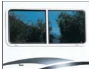
Optional "Stormtite" double glazed windows eliminate condensation and allow all season comfort. Solar reflective glass filters UV rays and reduces heat build-up in summer. By far the best made window in the RV industry.
